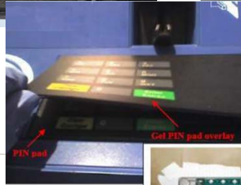
Reverse side of PIN pad overlay
